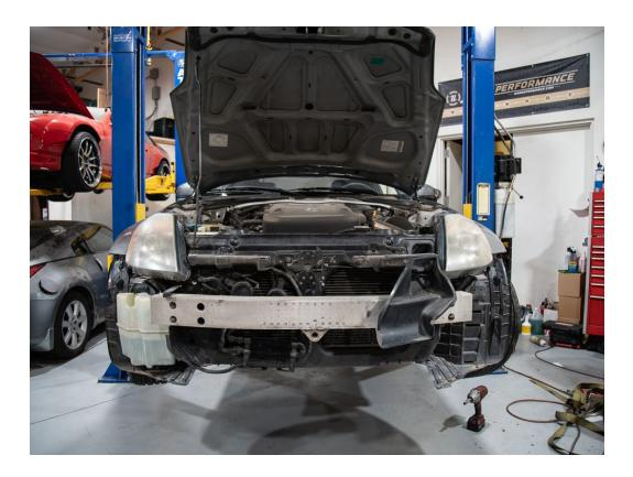
5. Disconnect the stock power steering cooler and drain the old power steering fluid.
