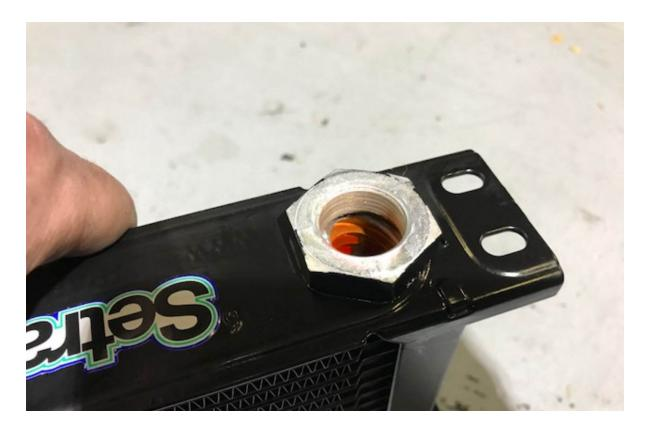
11. Apply a dab of fresh oil to the o-ring seal and thread the -6 AN to 22mm adapter fittings to the top of the cooler core and tighten them down.
