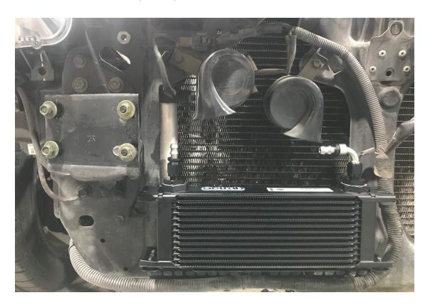
14. Attach the 3/8" oil hose to one of the stock oil cooler hard lines that we removed the clamps from in step # 7 and run it through the core support to the straight -6AN push-on fitting on the cooler core and cut it to length. Install it fully onto both sides reusing the stock clamps on each end. Route the remaining line from the 90 degree fitting to the other stock power steering hardline and trim it down to the correct length if necessary, making sure to use the stock clamps on both sides.
