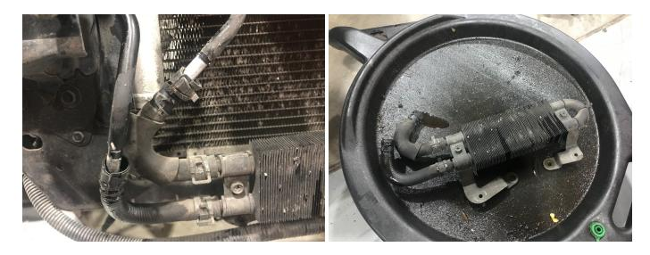
6. **For 350Z/G35's with the VQ35DE:** Remove the coolant overflow tank if it's in the way of your power steering lines, as we are removing the last section of the stock power steering cooler hard tubes that go through the core support
