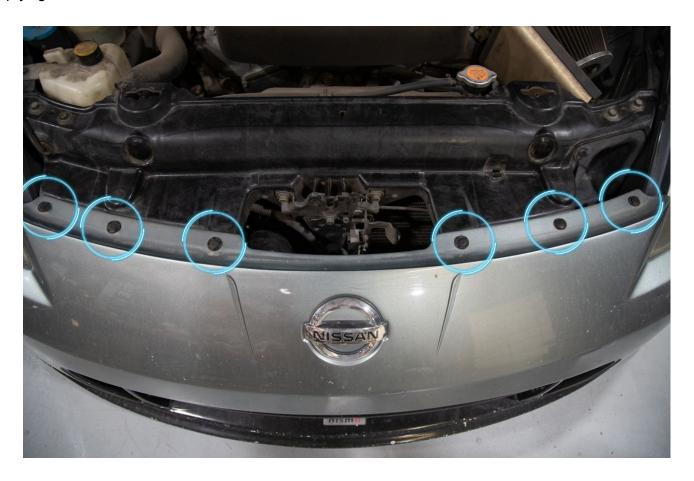
3. Lift the car and remove the 10mm bolts (Red: Bolts) and plastic pop-in clips (Blue: Pop Clips) along the bottom of the bumper cover and fender splash shields that hold the under tray in place.
