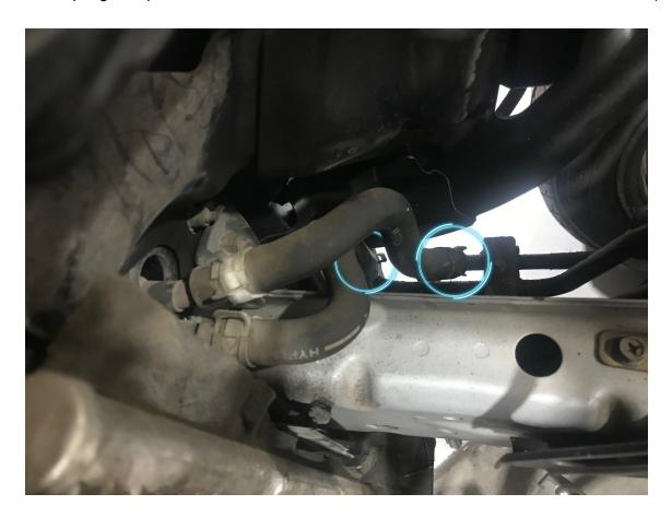
8. Remove the 10mm bolt securing the bracket that is holding the lines to the front core support, snip the zip tie holding it together and remove the bracket and rubber grommet as well as the two hard lines it was used to secure.
