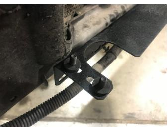
13. Attach the -6AN push-on fittings with the straight fitting on the outer side and the 90 degree fitting on the inner side pointed towards the other fitting and tighten them both down.
