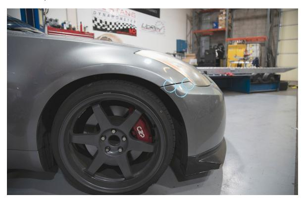
With the wheel turned inwards slightly, you can push the fender liner out of the way slightly and gain access to the two bolts going up into the fender and the one bolt going upward, mounting the bumper bracket to the headlight. All three are 10mm and may require the use of an extension.(Repeat for both sides)
