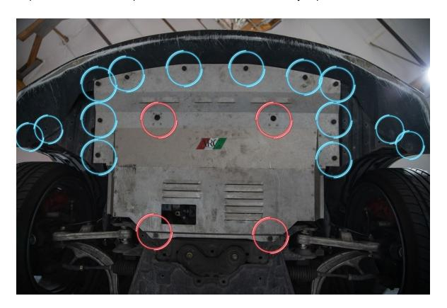
4. Carefully remove the bumper cover. With two people, gently pull the bumper cover forward and away from the body of the car. Removing the aluminum crash bar is not necessary but does free up space and makes the install easier.
