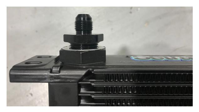
12. **For 350Z:** Mount the cooler to the 2 factory oil cooler M6 mounting holes using the two longer M6 bolts making sure to place the aluminum M6 spacers between the core support and the bracket to space it out from the factory bulge that is molded into the core support for the receiver dryer tank.
